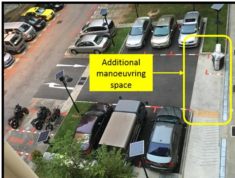
Fig. 4.4a Increase manoeuvring space for end lots
