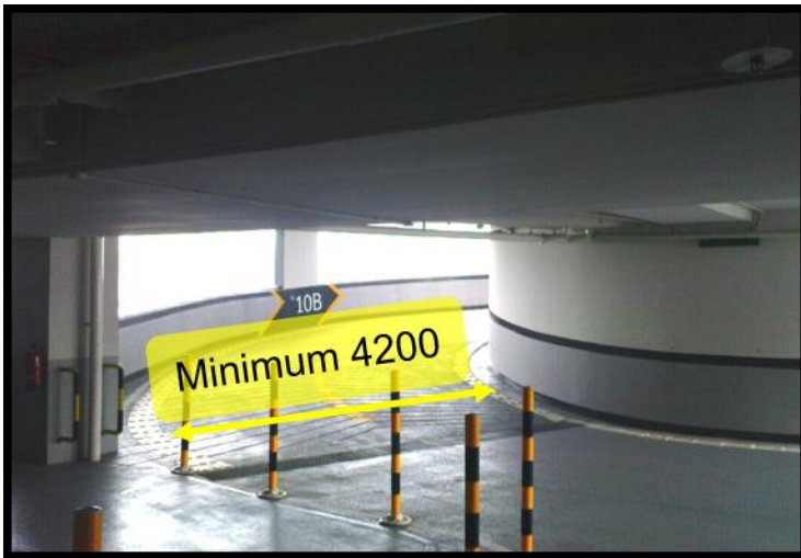
Fig 2.1.3g Example of a single, curved lane
