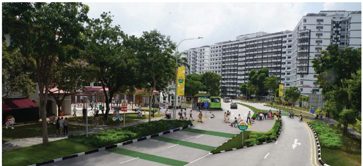
Upgrading and relocation of bus stop fronting Block 484 to cater for new kerb-less crossing between the Neighbourhood Centre (Central Courtyard) and Residential Cluster (Butterfly Walk)
