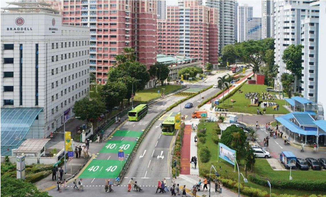
Street signs, green road surface markings and road humps when entering and driving along Friendly Streets to remind drivers to slow down
