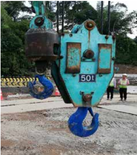
Load hooks with swivel and safety latch
