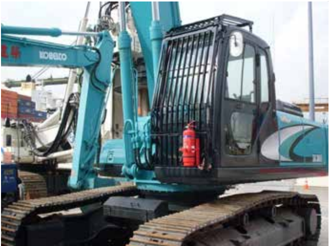
Excavator with reinforced roof
