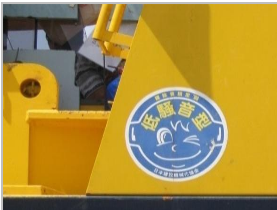
Use of sound-reduced machinery
