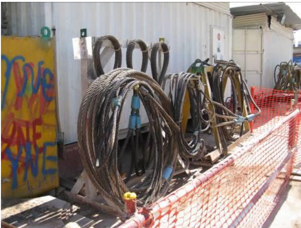
Lifting gears properly stored and maintained in good condition
