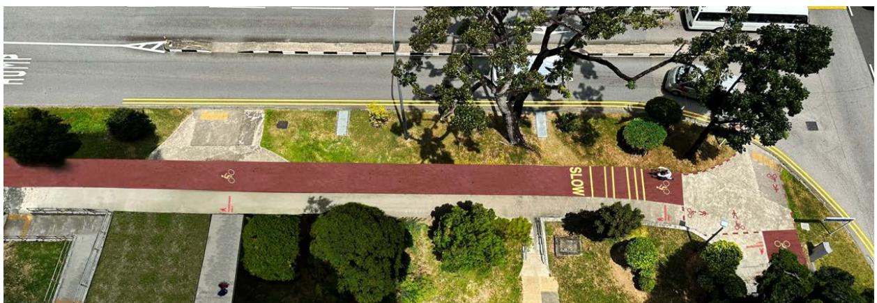
For illustration purposes only – Pedestrians-Only and cyclist logos at regular intervals of Pedestrian-Only Path and dedicated cycling path.
