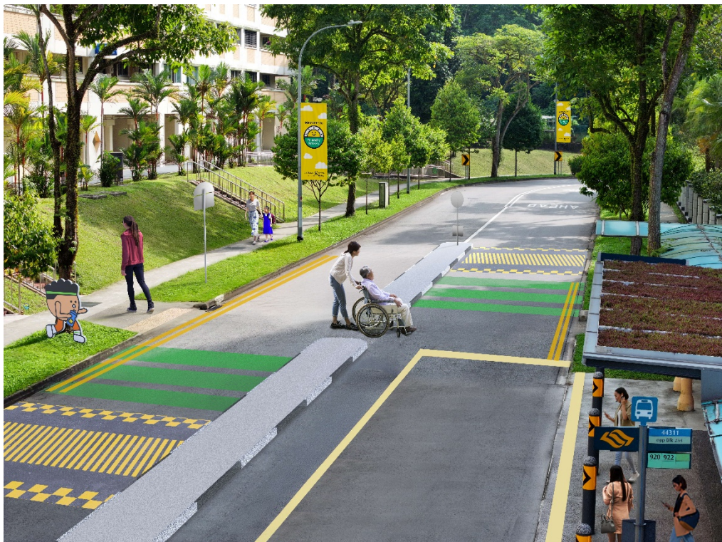
New bus-friendly humps to slow down traffic and wider centre medians and kerbless crossings for safer crossings
